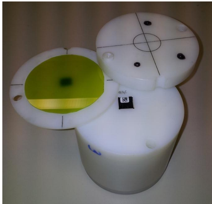
Figure 3.2: Cylindrical insert. The insert is separated into multiple compartments: a film plate and two OSLDs at 1.5 cm and 7.5 cm depth each.
