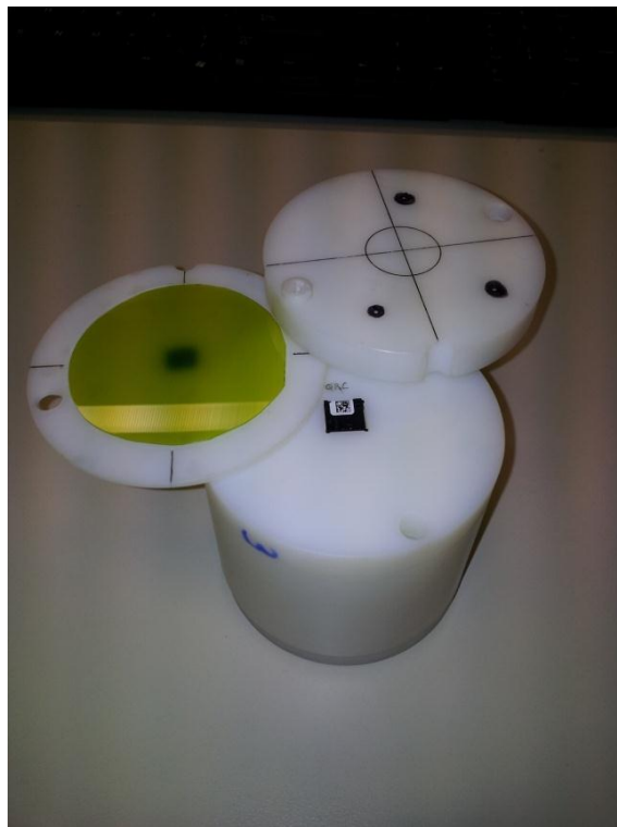
Figure 1: Film and OSLD cylindrical insert
