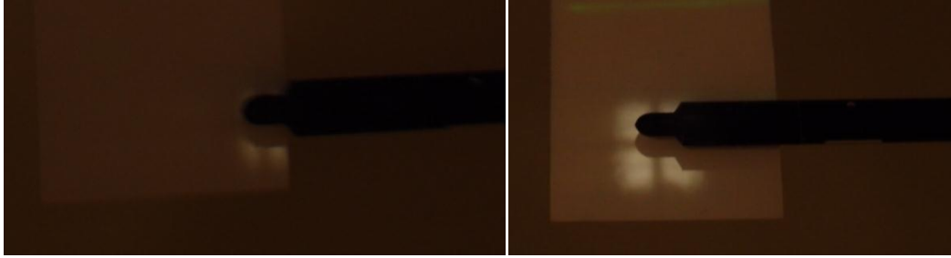
Figure 2.10: Exradin A16 with two field sizes superimposed. Left – 0.6 \times 0.6 \text{ cm}^2 . Right – 1 \times 1 \text{ cm}^2 .
