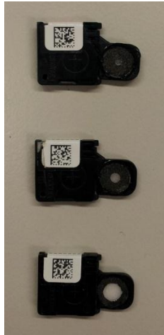
Figure 2.3: Masked OSLDs with 1mm (top), 2mm (middle), and 3mm (bottom) diameter masks.
