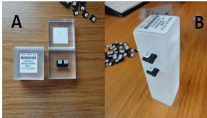
Figure 1.2: Examples of two acrylic miniphantoms used by the RPC as a remote audit tool for external beam. Miniphantoms for photons (A) and electrons (B) are shown.
