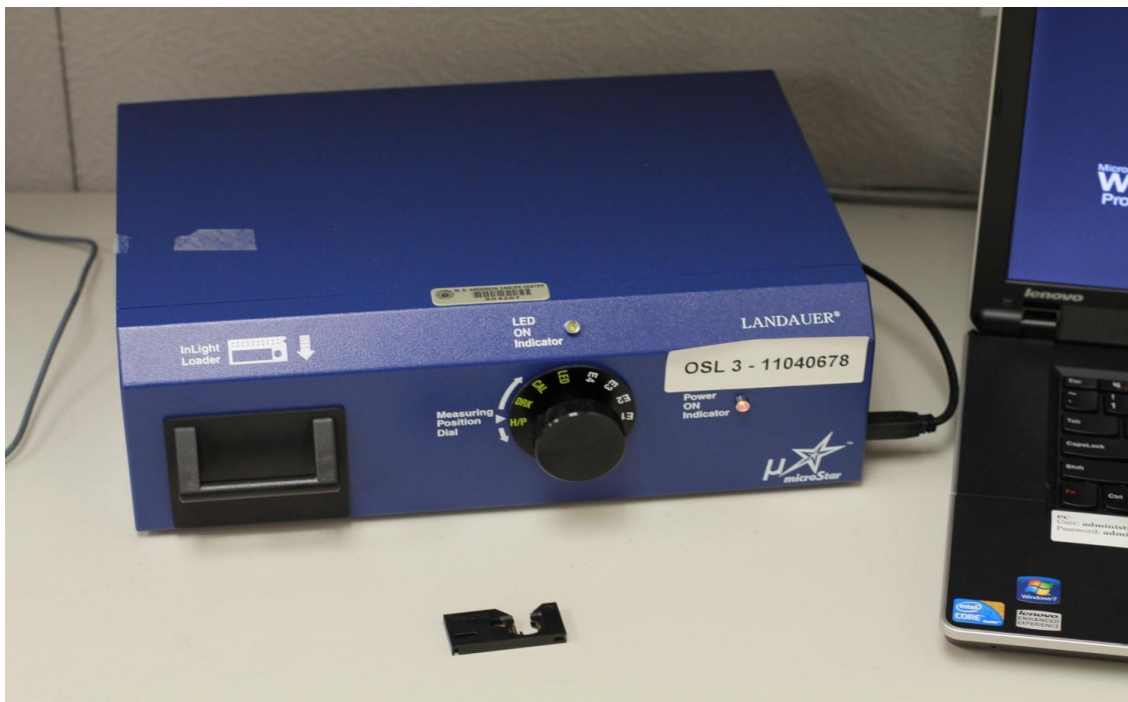
Figure 2.7: Landauer’s microStar reader with holder. nanoDots are loaded into the holder and placed inside the black tray. The readout process commences once the knob is turned.
