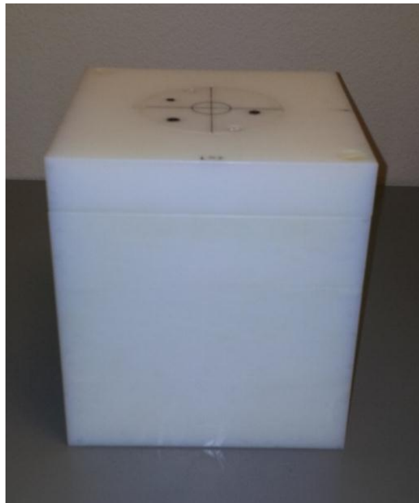
Figure 3.1: Full phantom prototype. The phantom is comprised of a lid, base, and cylindrical cone and houses four OSLDs at two depths and a film insert.
