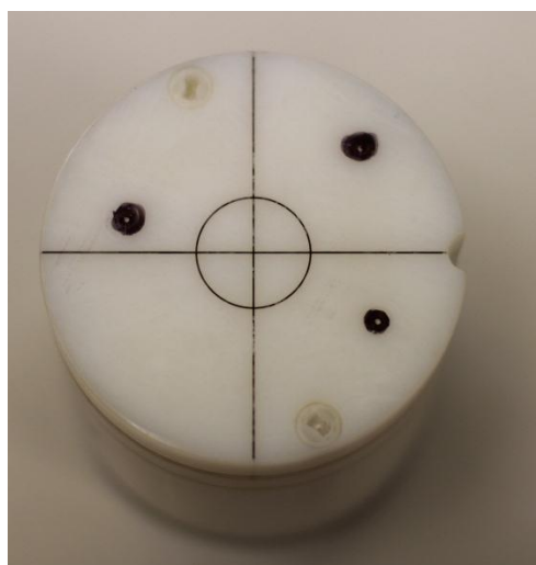
Figure 2.1: Cylindrical insert with pin prick holes used for film localization.
