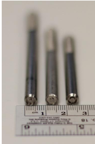
Figure 2.5: Hole punching tool used to create various sized masks. From left to right: 1 mm, 2 mm, and 3 mm.
