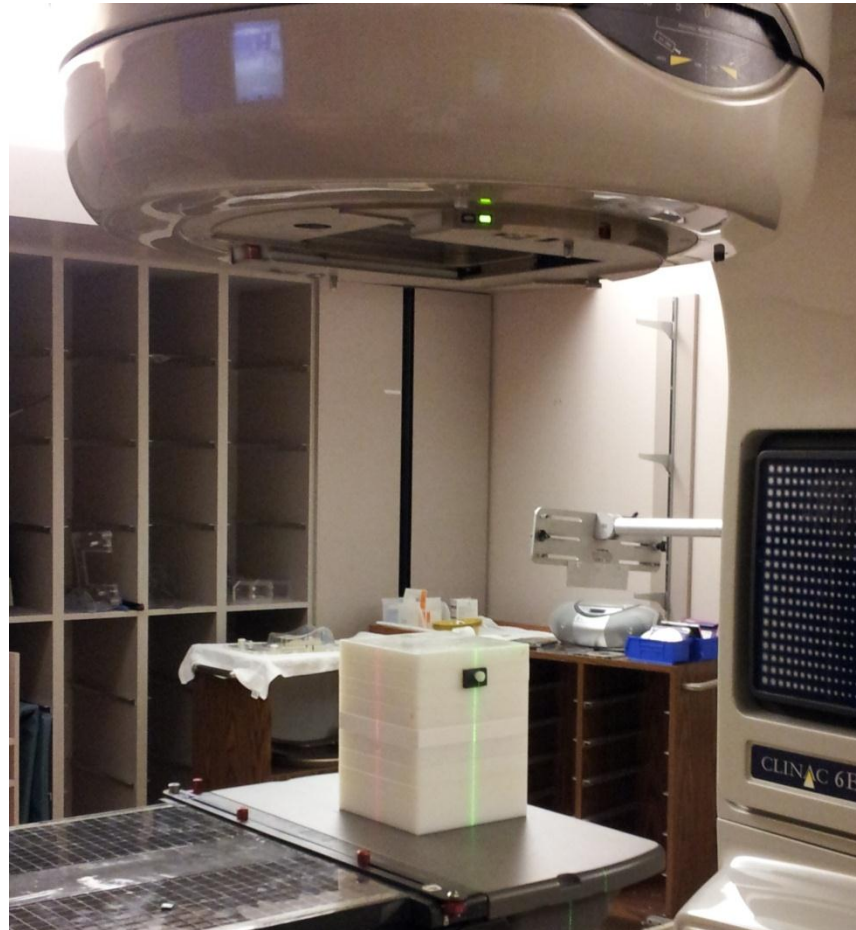
Figure 2.6: Reproducibility setup. Each dot is placed in the removable grey insert. Irradiations are performed for each mask and at four different doses.
