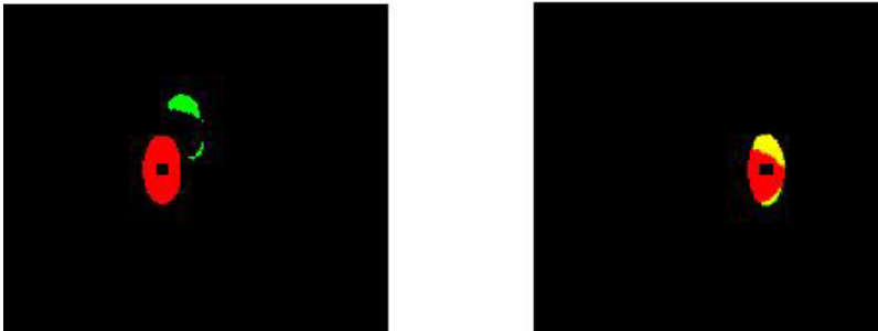
Figure 26: Missing Information test: Successful Registration with only 25.3% of the object visible (left) before registration with HD mean: 9.12 mm and (right) after registration (HD mean: 1.92mm after registration)
