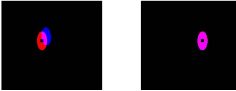
Figure 27: Test Objects Demonstrating successful registration; (left) Before (HD mean: 3.99mm) and (right) After Registration (HD mean: 0.67mm)
