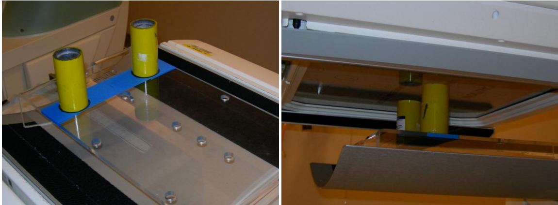
Fig. 6-3A (left) and B (right). Photographs of the experimental set up for evaluating image distortion are shown here. Sources are positioned at a fixed distance for the duration of the experiment.
