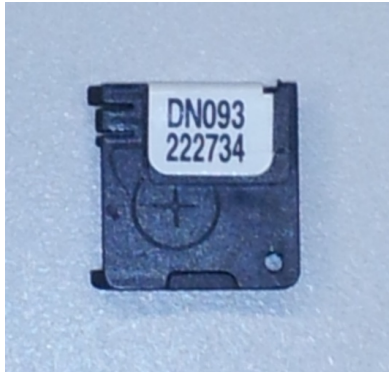
Figure 2.12 nanoDot OSLD from Landauer, Inc.
