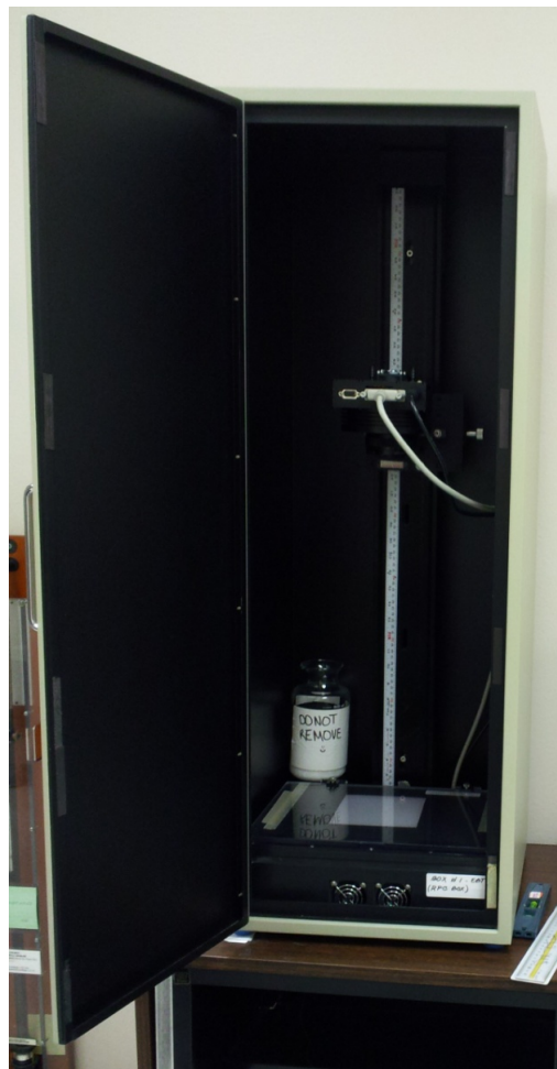
Figure 2.15 Setup of microdensitometer used for film scanning
