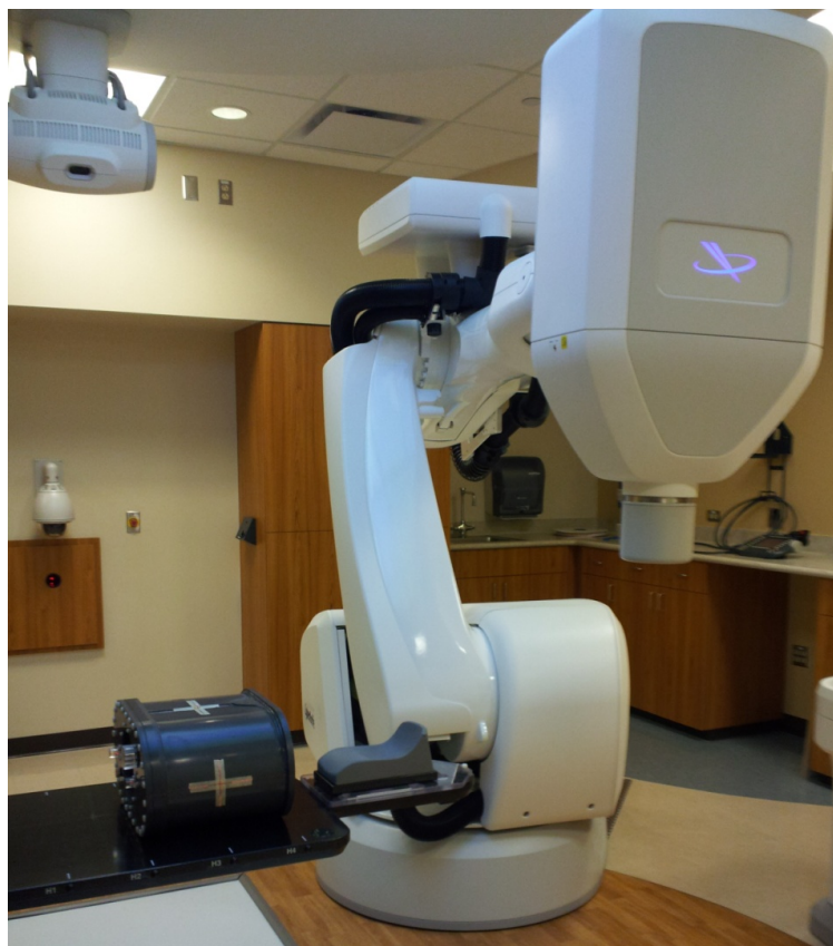
Figure 2.11 CyberKnife irradiation of pelvic phantom
