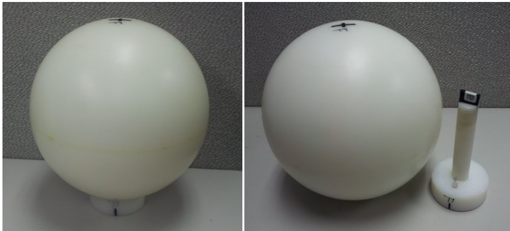
Figure 2.1 High-impact polystyrene spherical phantom (left), and phantom base and insert holding the OSLD within the spherical phantom (right)
