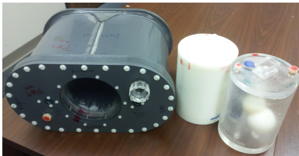
Figure 2.3 RPC pelvic phantom shell (left) with dosimetry (middle) and imaging (right) inserts
