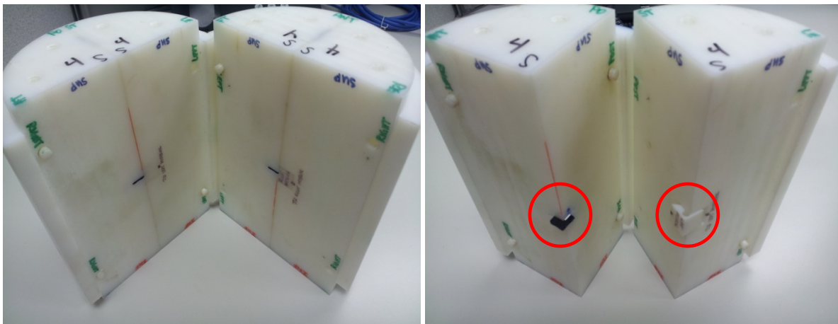
Figure 2.4 Dosimetry insert split into posterior and anterior half (left), and posterior half split into two quarters to show positioning of OSLD and TLD (red circles) at the center of the target (right)
