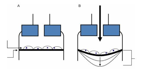
Figure 2.1. Cell Injury Controller II. A. Brain microvessel endothelial cells are grown on an elastic membrane. B. Mechanical stretch is applied by a short (50 ms) injection of nitrogen gas, which deforms the elastic membrane. mmol/L): 140 NaCl, 5.4 KCl, 2 CaCl<sub>2</sub>, 0.5 MgCl<sub>2</sub>, 0.4 MgSO<sub>4</sub>, 3.3 NaHCO<sub>3</sub>, 10 HEPES, 5.5 glucose, and pH of 7.4. A calcium-free MBSS solution was also utilized containing 1 mmol/L EGTA in place of 2 mmol/L CaCl<sub>2</sub>.
