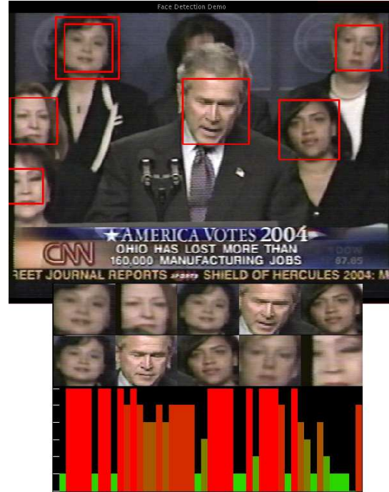
Figure 5: Face Detection, Extraction and Temporal Density Plots. Top – an image from video with faces marked. Bottom – density of faces over time (left to right) in a stream.
