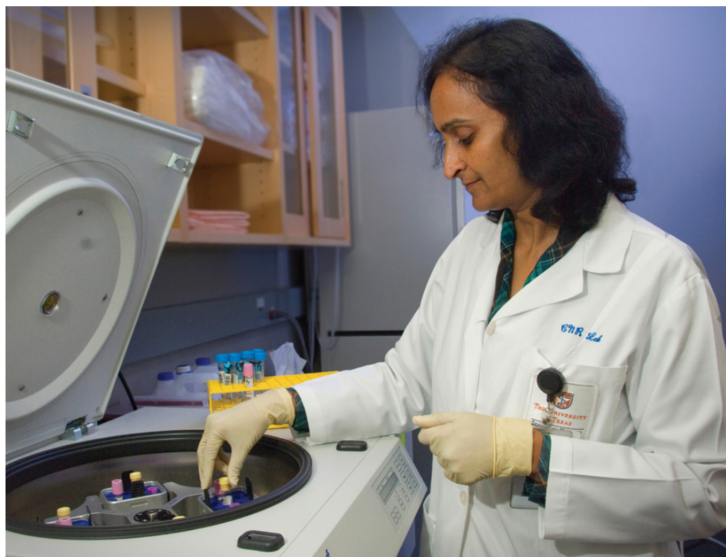
Malini Udtha, Ph.D., processes patients' samples for separation of blood components using the Biobank lab's ultra-centrifuge equipment.
