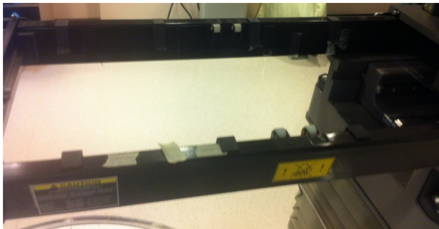
Figure 2-6. Movable support rails on Varian Exact Couch
