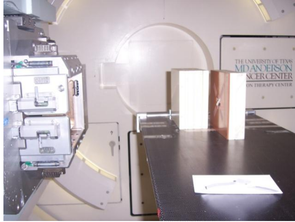
Figure 2.15 Side view of proton OSL/TL irradiation.
