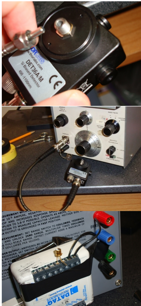
Figure 20: Photodiode module (top), electrometer (middle), and analog-to-digital converter (bottom) for converting emitted light into a digital signal
