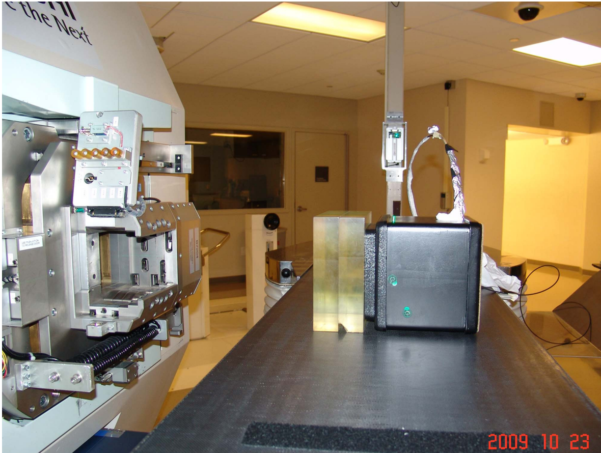
Figure 26: Experimental apparatus for measuring the photocurrent as a function of SOBP depth
