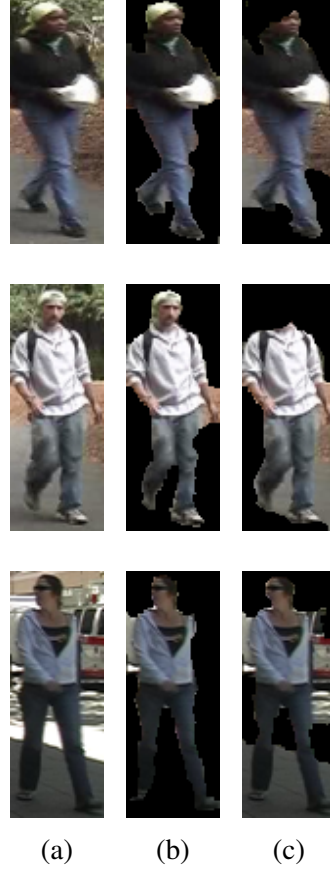
Fig. 2.2: Example outputs of foreground - background segmentation (a) Original image, (b) segmentation result with the proposed approach, (c) segmentation result with the approach in [2].
