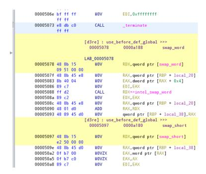
**Figure 3.7:** Ghidra with highlights and comments declaratively specified to output results inferred via D3RE for our example
