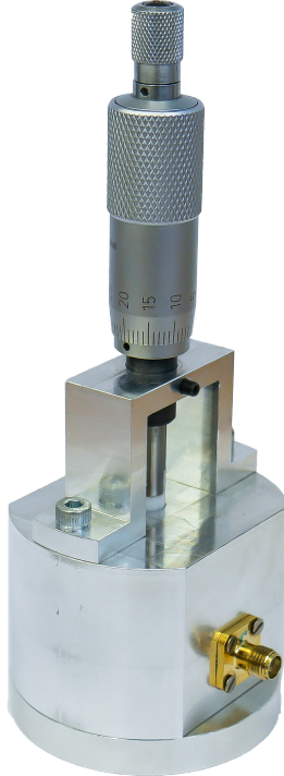
Figure 3.5: Photograph of the lift off dielectric resonator fixture. Reprinted from [91] ©2021 IEEE.
