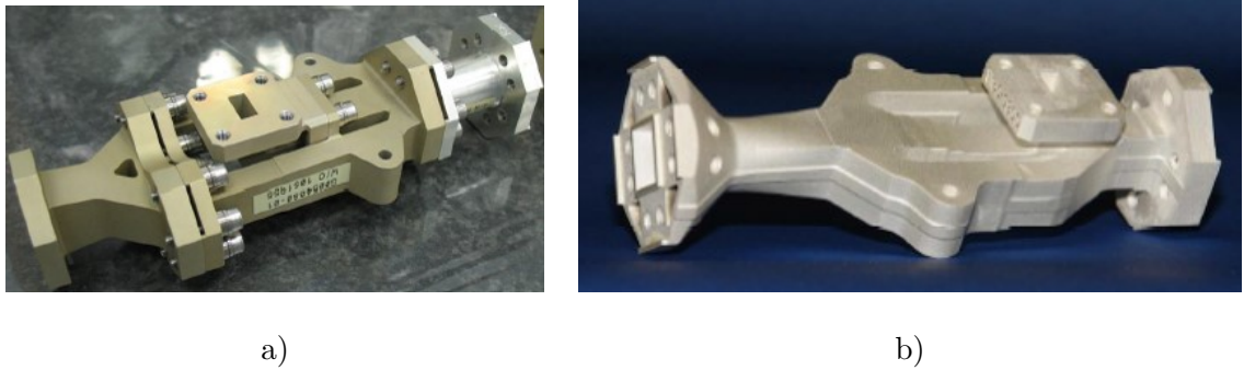
Figure 2.5: Ortho Mode Transducers produced by a) multi part traditional manufacturing and b) monolithic additive manufacturing. Reprinted from [39] ©2017 IEEE.
