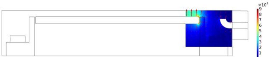
Figure 3.31: Cross section of the parallel plate resonator geometry, showing the coupling probe orientated parallel to the cavity wall as to align with electric field between the reference plate and the sample. Reprinted from [23] ©2021 IEEE.
