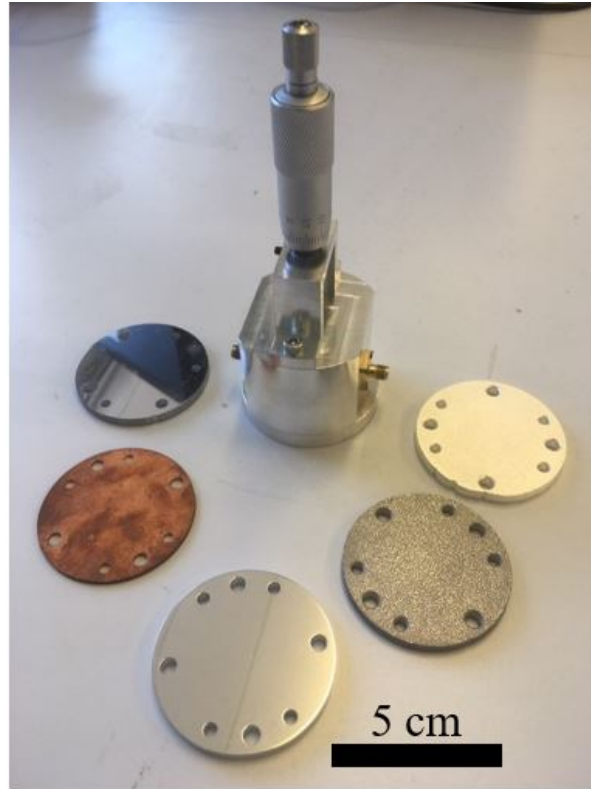
Figure 5.1: Photograph of the lift-off dielectric resonator fixture with samples plates of copper PCB and polished aluminium along with powder bed fusion samples treated by silver plating, media tumbling and machine polishing. Adapted from [25] ©2019 IEEE.
