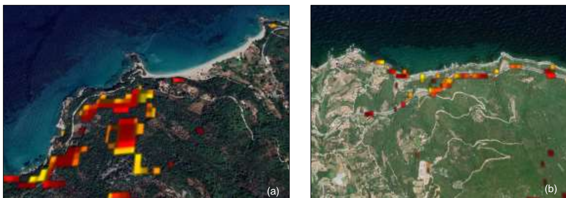
Figure 38: Damage Proxy Map (DPM) of Potami close to Karlovasi and Kontakeika (from the Advanced Rapid Imaging and Analysis (ARIA) Centre for Natural Hazards, https://aria-share.jpl.nasa.gov/20201030-Samos-Izmir-EQ/DPM/ ). The colour grading from yellow to red indicates increasingly higher ground deformation.
