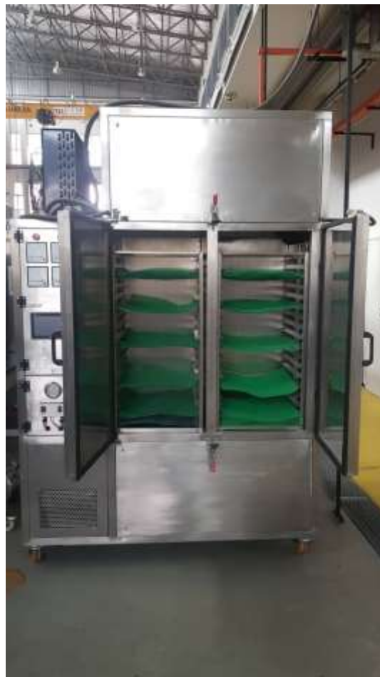
Figure B2 Actual diagram of inner compartment of heat pump dryer
