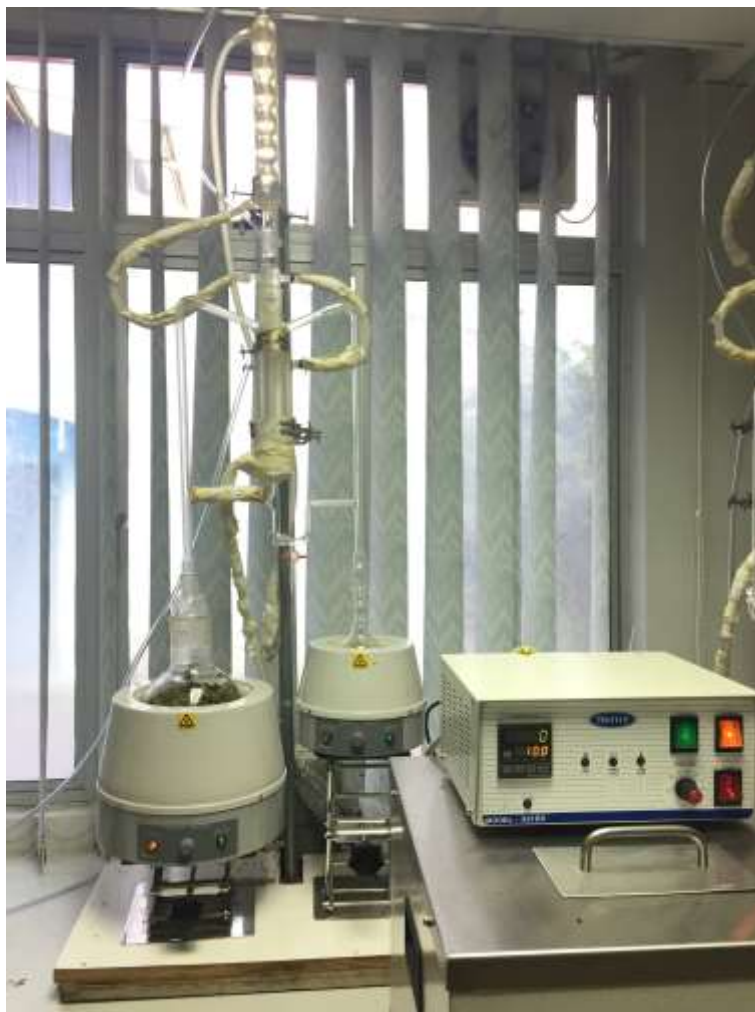
Figure 3.8 Simultaneous distillation and extraction (SDE) unit with refrigerated water circulator
