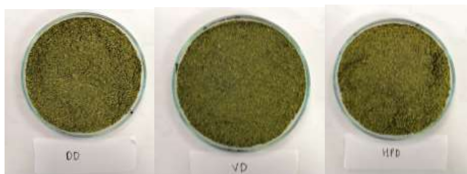
Figure 3.6 Milled dried lemon myrtle leaves of (a) oven dried; (b) vacuum dried and (c) heat pump dried
