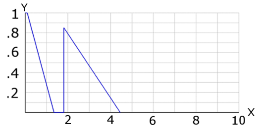
(d) Embedded set determining the right-endpoint of the type-reduced set of the IT2 set in Fig. 7.7a (EIA)
