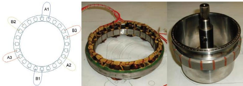
Figure 2.23 Nose wheel actuator motor [78]
