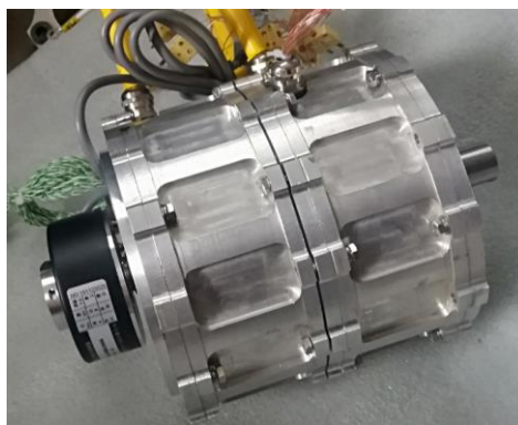
Figure 8.24 Two interconnected EMA motors assembled together
