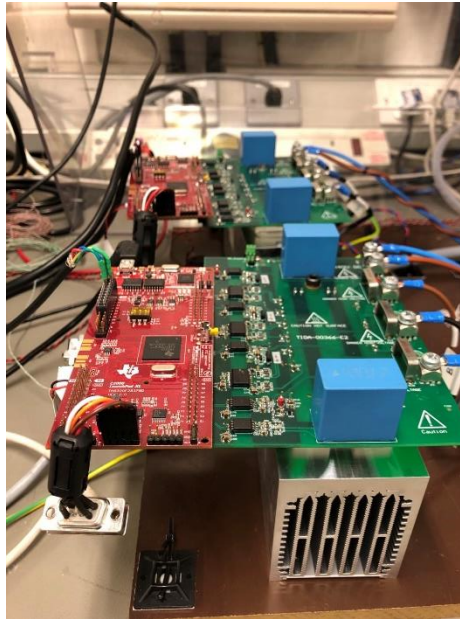
(a) Back-to-back 3-phase voltage source inverters (VSI)
