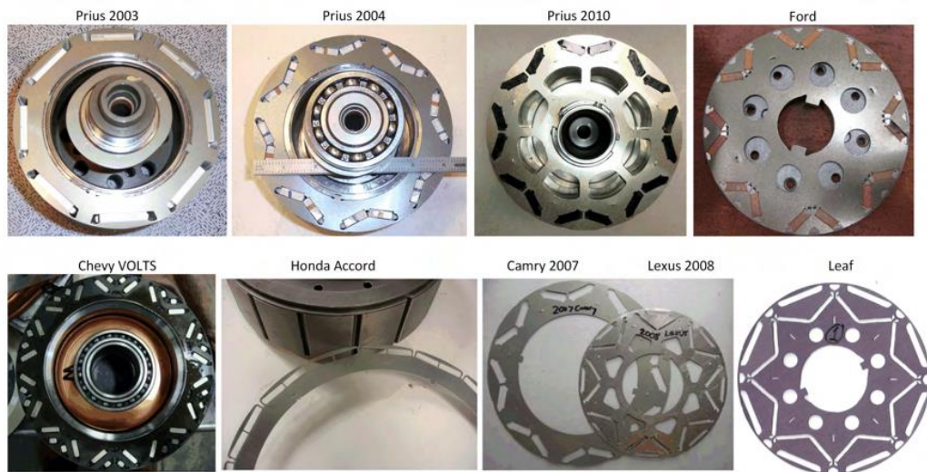
Figure 2.3 Rotor of different PM synchronous motors [24]-[27]
