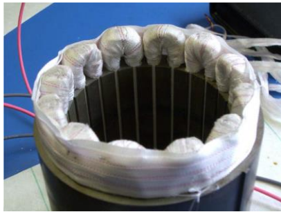
(a) Stator with concentrated winding
