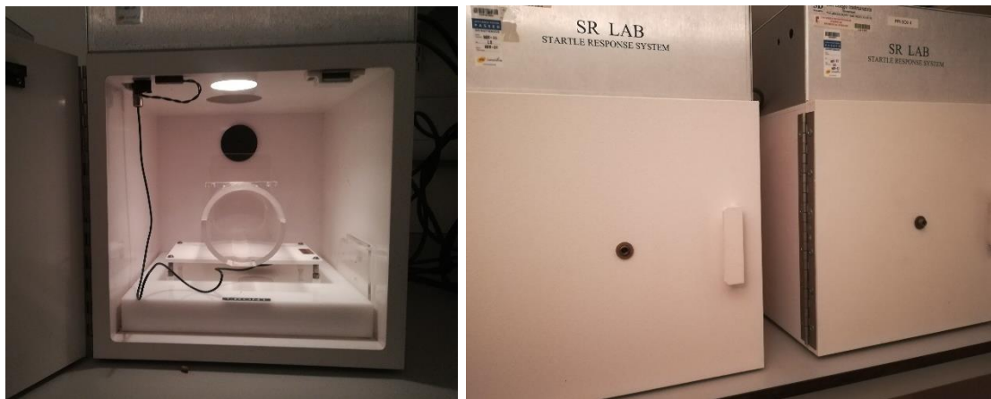
FIGURE 2.4. – STARTLE/PREPULSE INHIBITION CHAMBER USED TO MEASURE SENSORIMOTOR GATING. Rats were placed in a Plexiglas cylinder inside a sound-attenuated chamber. The cylinder was linked to an accelerometer to measure the startle response to the different pulse intensities presented during the test.
