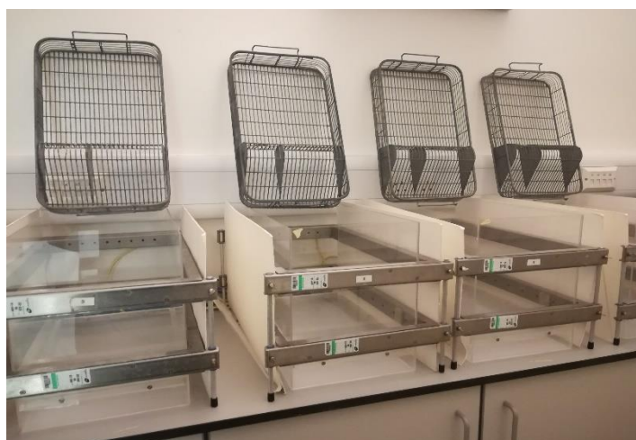
FIGURE 2.3. – OPEN-FIELD CHAMBER USED TO MEASURE LOCOMOTOR ACTIVITY. Rats were placed in Plexiglas chambers for 30 minutes and locomotor activity was measured by break of photobeams.
