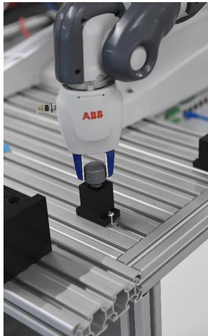
*Figure 4.1: Experimental setup for the bolt tightening subtask.*
