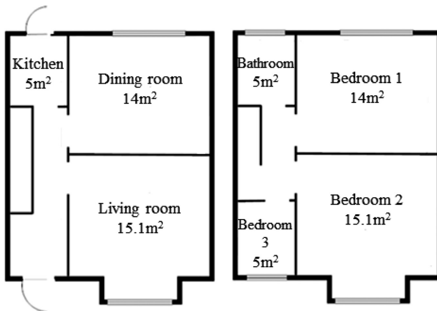
Fig. 4. Floor plans of the reference house used to test zoning strategy and geometry simplification (left: ground floor, right: first floor).
