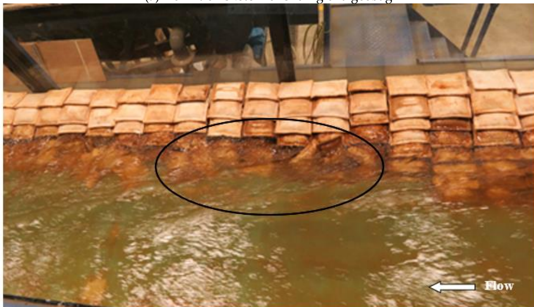
(b) Sliding of geobags in high-water level condition, side slope 1V:2H
