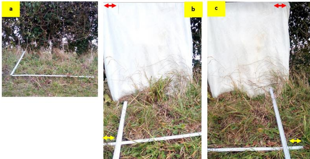
Figure 4.33a - c: Process of establishing a white background for 1 m hedgerow samples. a = Sample without white background. b & c = Using the meter rule and marker to remove 10 cm of white background from right and left side. Red arrows portray 10 cm on white sheet. Yellow arrows portray 10 cm on meter rule.
