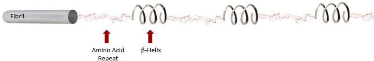
Figure 2.3d: Schematic diagram of secondary molecular structure of the flagelliform silk fibril (Adapted from writings of Ayoub et al. (2007), Craig (2003) and Hayashi & Lewis (2001)).
