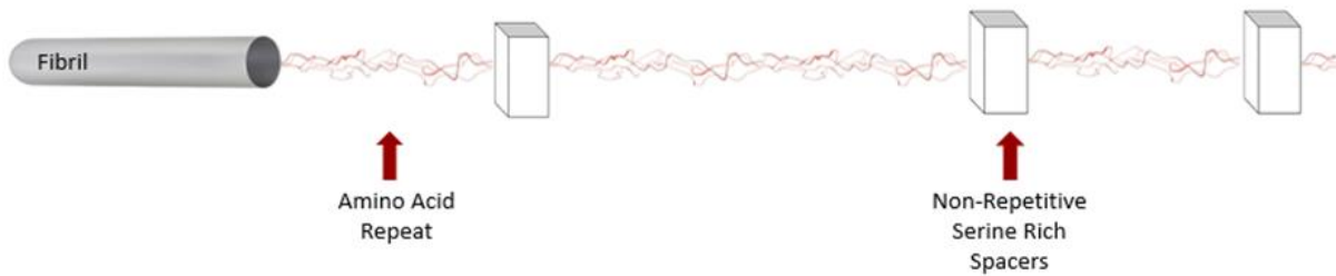
Figure 2.3b: Schematic diagram of secondary molecular structure of the minor ampullate silk fibril (Adapted from writings of Basu (2015), Craig (2003), Rising et al. (2005) and Tokareva et al. (2014)).
