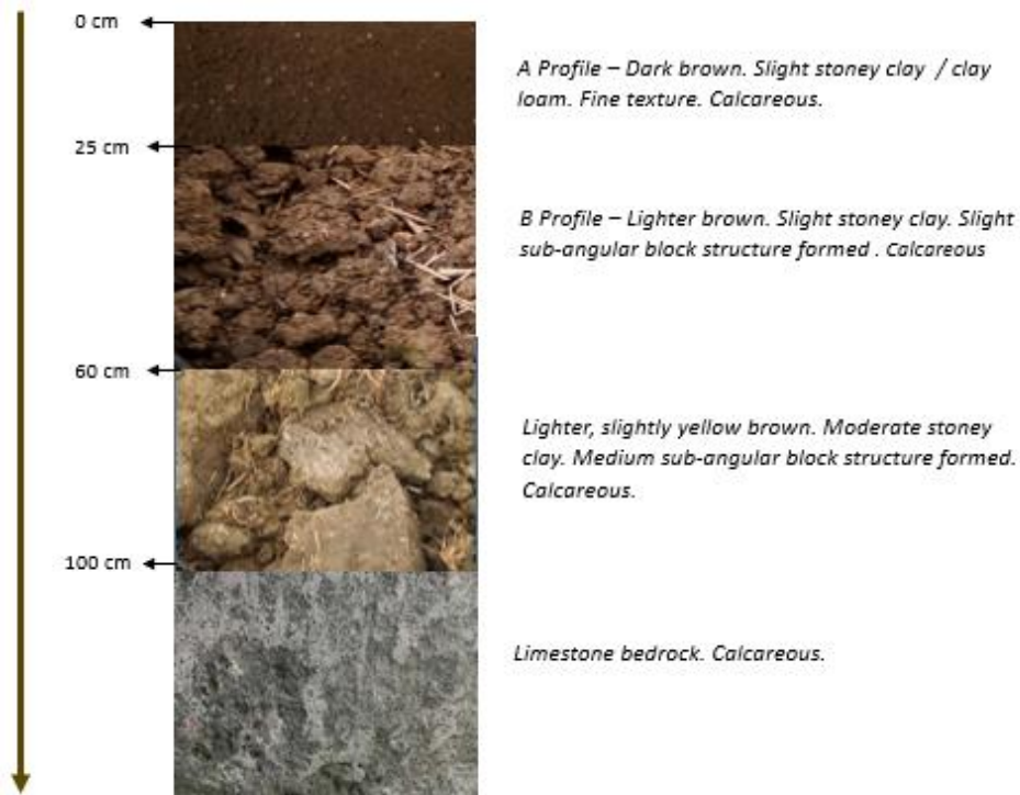
Figure 3.4: Schematic diagram showing soil profile of Hanslope soil series 4.1 (Adapted from Cranfield University 2017).
