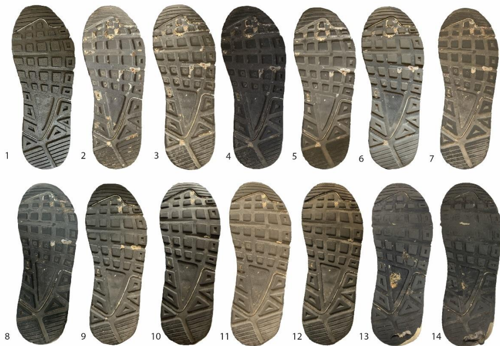
Figure 2. A visual timeline of features of footwear on the same size 9 men's unbranded trainer worn for a period of 3 months. Note the wear features appearing rapidly and large RACs appearing towards the end of the series.
