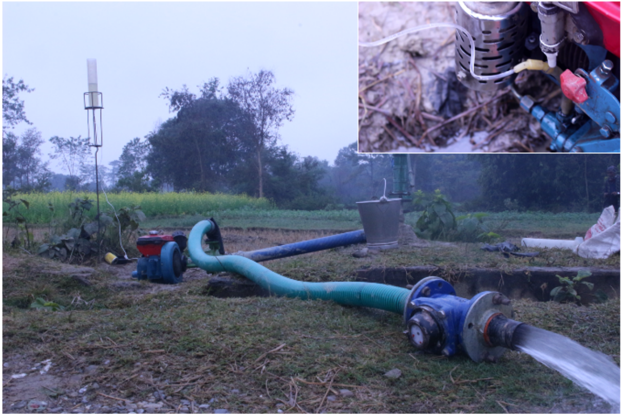
Figure 3. Setup of pump testing rig during one of the 116 in-situ tests conducted as part of this study. Inset image shows a close-up view of the fuel injection from the graduated measuring cylinder into the pump engine.
