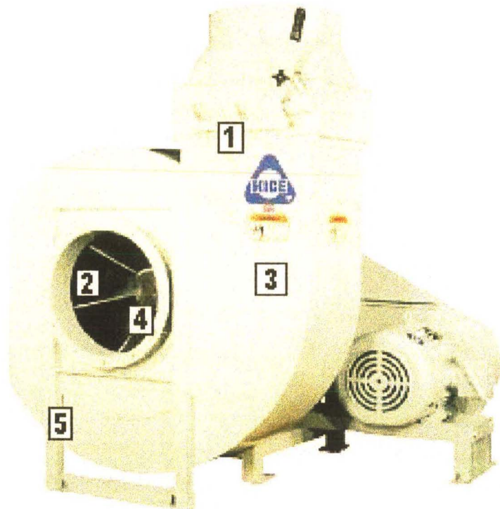
Fig. 2.9 Centrifugal fan showing, air outlet (1), impeller (2), spiral shaped casting (3), air inlet (4), framework (5) [8].
