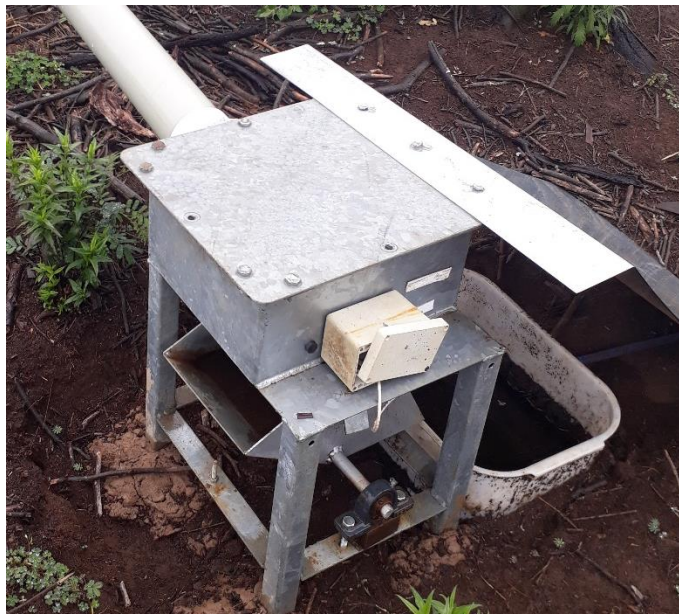
Plate 3.8: Tipping bucket gauging system for measuring surface runoff.
