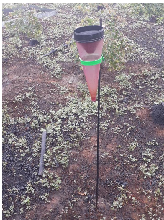
Plate 3.3: Manual rain gauge installed at the research location.
