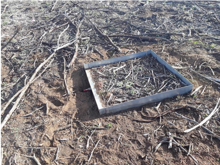
Plate A-9: Mulch treatment micro-runoff plot setup.
