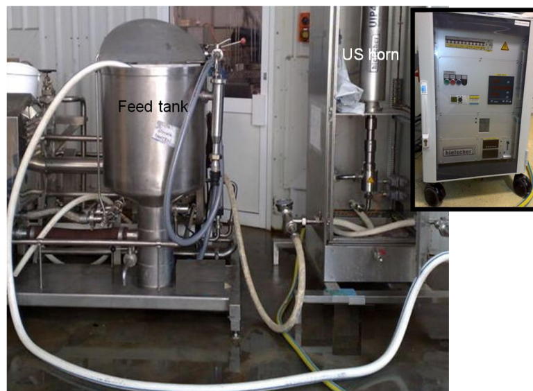
Fig 1. Pilot-scale experimental setup used in dairy processing using Hielscher Systems GmbH UIP-400 (Figure Adapted from [11])
