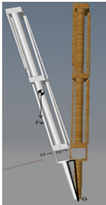
Figure 4.18 FBD Joint 3: This is a side view of the pile, focusing on the forces on Joint 3.
