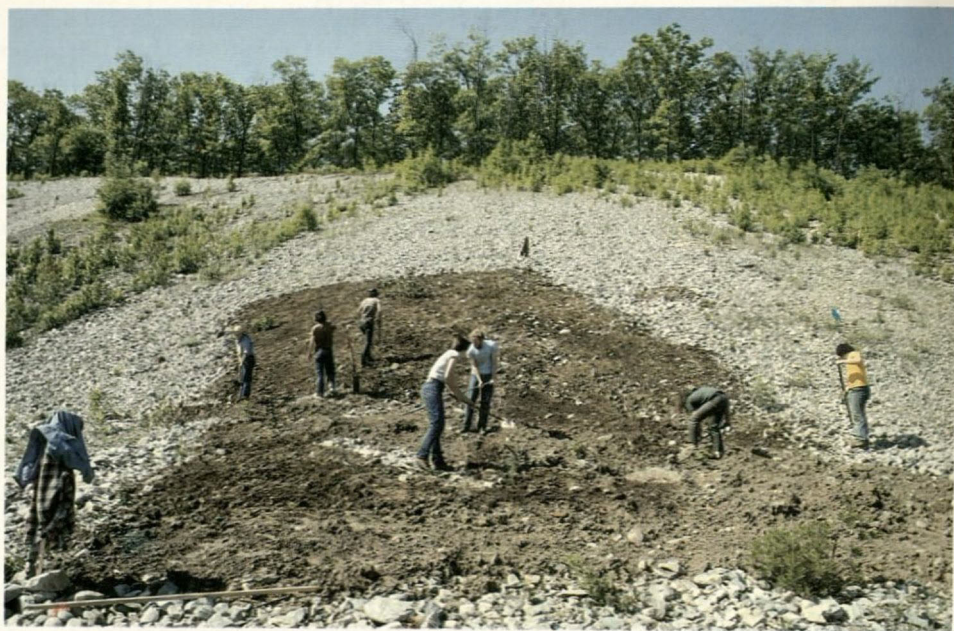
Fig. 1. Application of fresh mycelium-soil mixture on experimental plot, north-facing slope of gravel pit (May, 1976).
