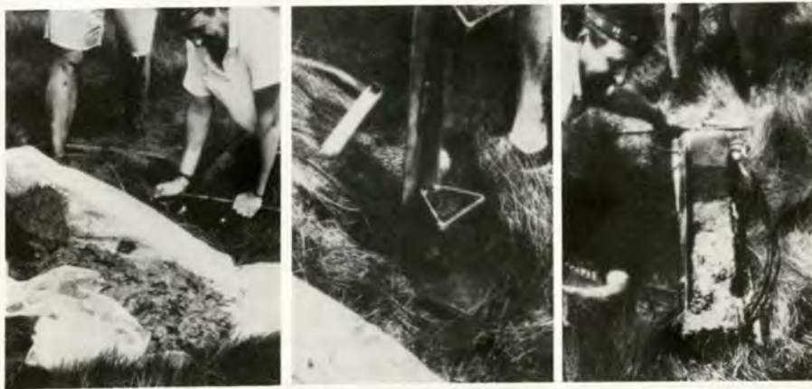
Fig. 1. Sequence showing steps in obtaining a peat core with modified McCaffrey sampler. Left—Hole is being excavated with post hole auger. The surface block of grass turf shows to the left. Center—Cutting edges of sampler are placed on edge of hole with bottom door open and over the hole. Sampler is now ready to be pushed down along side of hole just excavated. Two foot braces to aid in the process are shown. Right—Sampler removed with section of peat. Three metal bands hold the peat against the metal frame while extracting.
