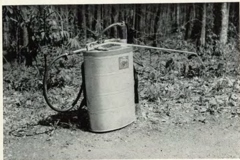
Fig. 7. A five-gallon back-pack sprayer of the type used by the U. S. Forest Service.
