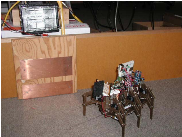
Fig. 1. The robot, its metallic probes, the power station, and the light source. Six pairs of capacitors are attached underneath to power the ServoBot.
