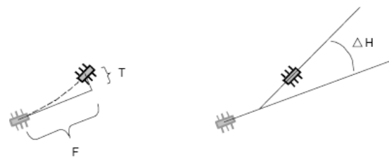
Fig. 3. Gait Cycle Turn Measurements. The left diagram shows F and T. F is the distance moved forward. T is the distance moved in the turn direction. The right diagram shows \Delta H , the change in heading [20].
