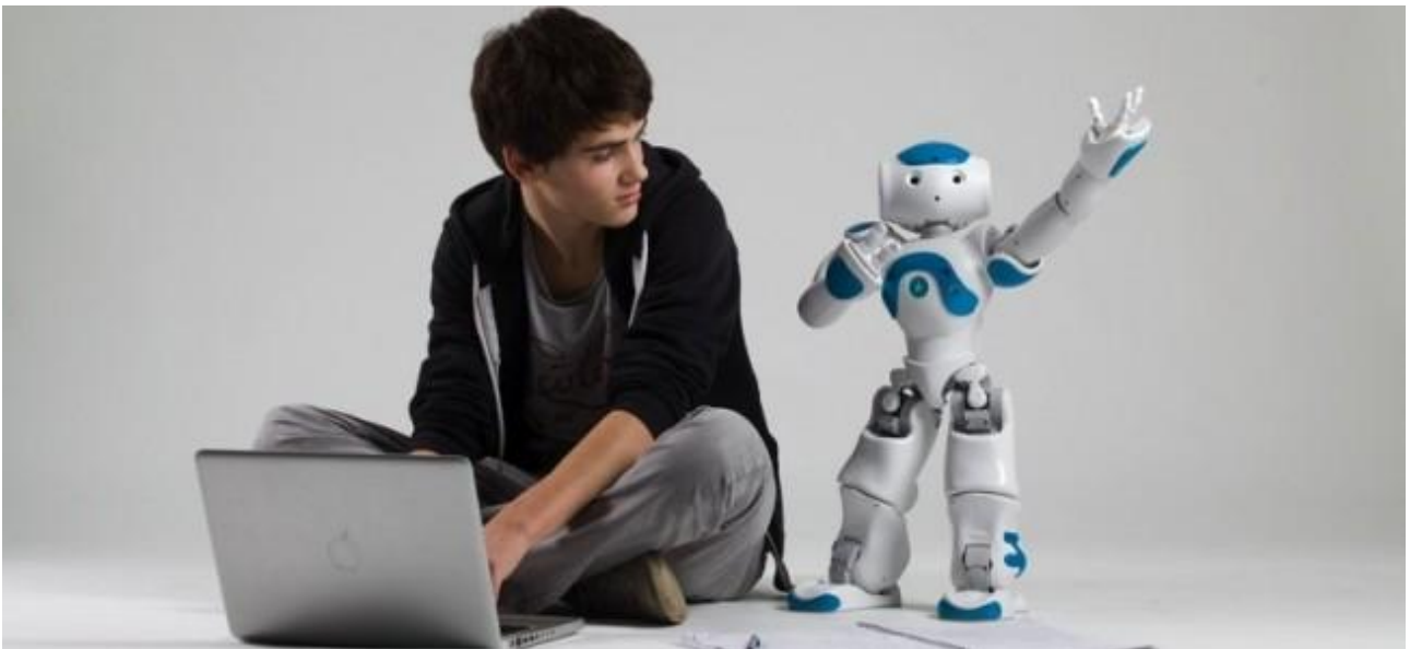
Figure 1. The Nao humanoid robot, by Aldebaran Robotics. Kadam and Sheng [8] used this robot for electroencephalographic teleoperation.
