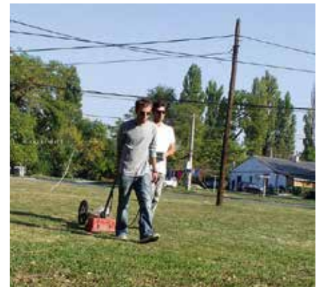
Figure 2: Ground Penetrating Radar (GPR) survey (Copyright: Dr Caroline Sturdy Colls)
