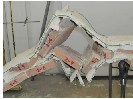
Figure 17 – Ring separation of the brick layers and GFRP reinforcement
