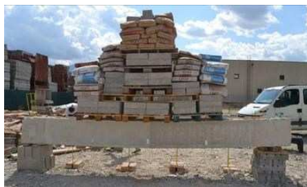
Figure 22 – Bending test set-up
