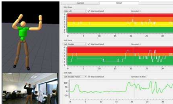
Figure 6: Example of ergonomics application based on our Kinect data correction framework.
