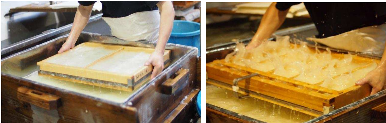
Figs. 1 & 2: Handmade Tamezuki process, Awagami Factory, To overcome the bias of causing fibres to orientate themselves parallel to the short side of the mould, the vatman shakes the screen between two perpendicular directions. This produces a sheet with no apparent directionality in contrast to Nagashizuki method Process and technical development of machine-made Japanese paper
