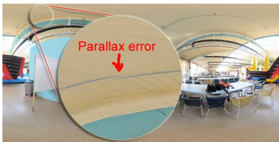
Fig. 2.6 Parallax effect error example in omnidirectional video. Taken from [34]
