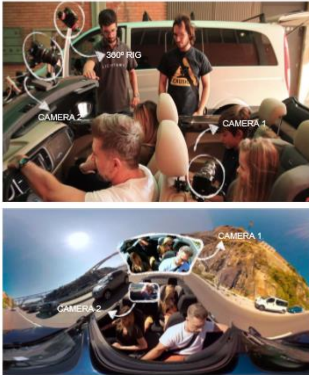
Figure 3: Top: a camera setup to record traditional and omnidirectional video simultaneously. Bottom: a schematic diagram of possible directive inserts located within the omnidirectional video. Image courtesy of Lightbox ( www.lightbox.pt ).
