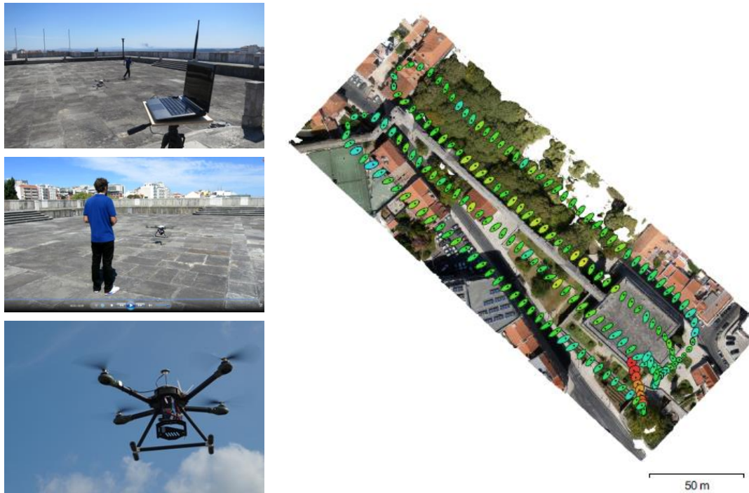
Figure 2 UAV data acquisition in Mãe de Água reservoir (Lisbon Aqueduct Structure): Setting the UAV flight plan (left) and camera locations (right).
