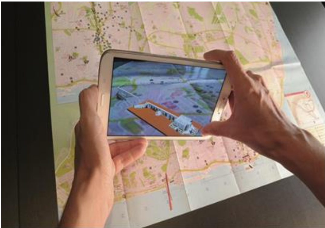
Figure 5. Mãe de Água reservoir 3D model and AR environments using the city map as a marker
