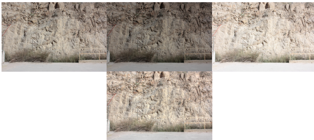
Figure 2. Image result (down) of combining three HDR images with different range of luminance (up)
