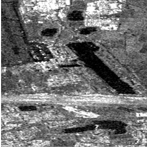
Fig. 14. Detail of the original COSMO-SkyMed image over Milano after resolution change and multi-looking (ML factor 50).
