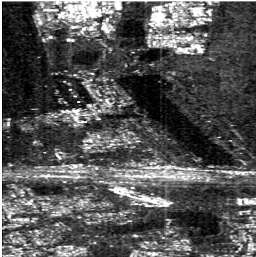
Fig. 15. Detail of the reconditioned GEOSAR demo product after clutter decorrelation (ML factor 50).
