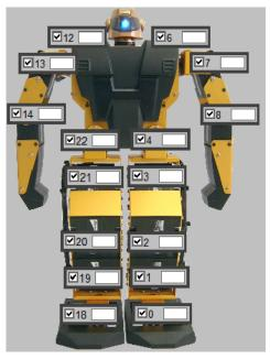
Fig. 1 Servomotors location at Robonova-I HITEC
