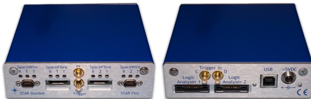
Fig. 3.1: The STAR Fire Mk2 Unit front panel (left) and bottom panel (right)
