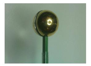
Figure 1. Photograph of the prototype of the spherical sensor anemometer.
