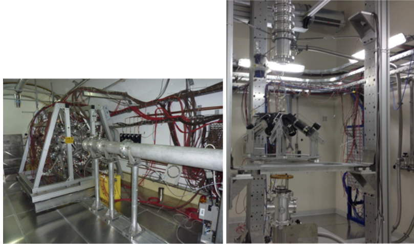
Figure 3. Total absorption calorimeter (TAC) in the n_TOF-EAR1 (left panel) and C 6 D 6 scintillators set-up in n_TOF-EAR2 (right panel). The horizontal and vertical beam lines are visible as well.
