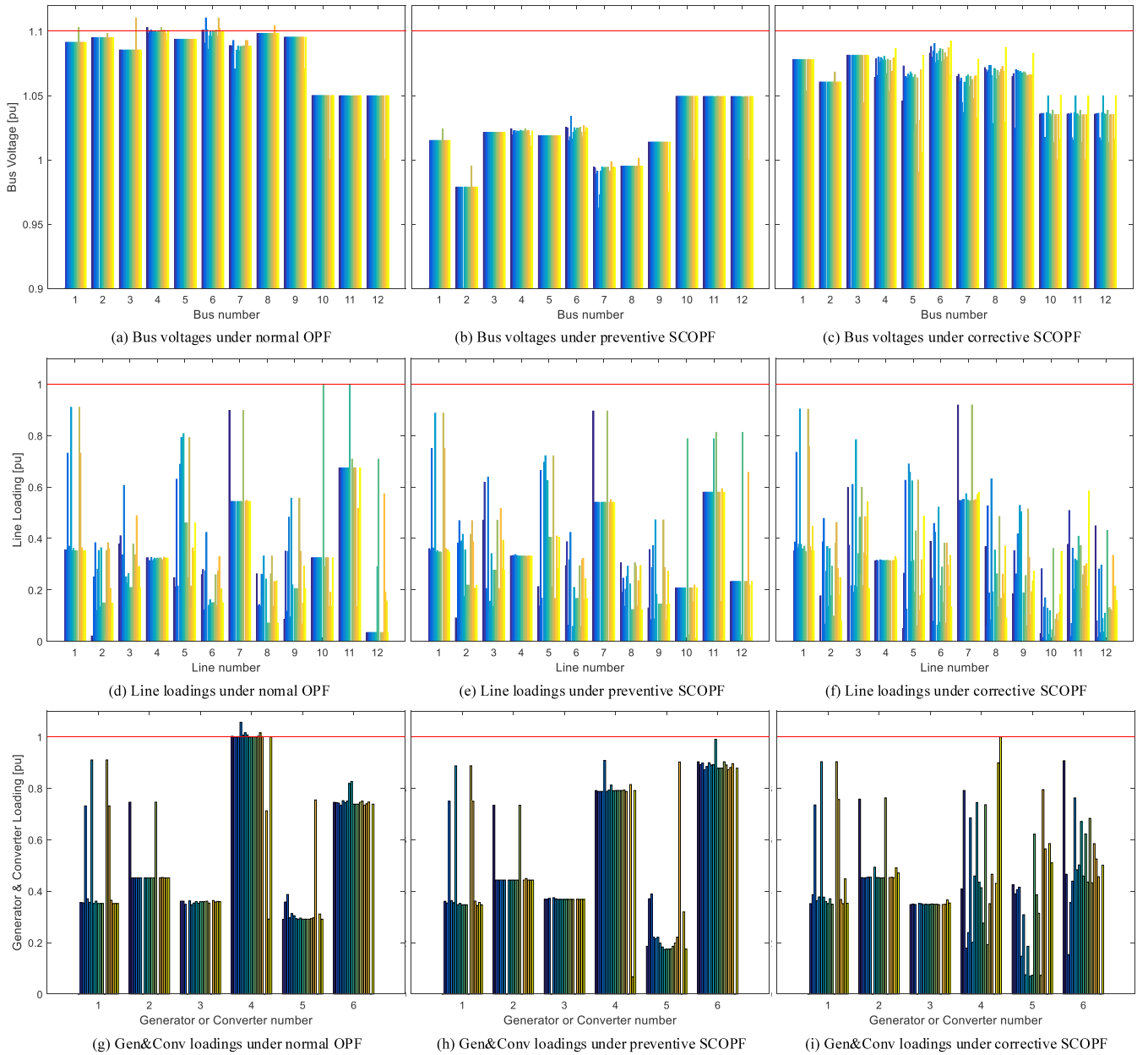
Fig. 5. Bus voltages, the generator loadings and the line loadings for the normal OPF, preventive SCOPF and corrective SCOPF operation for the 9AC+3DC network.
