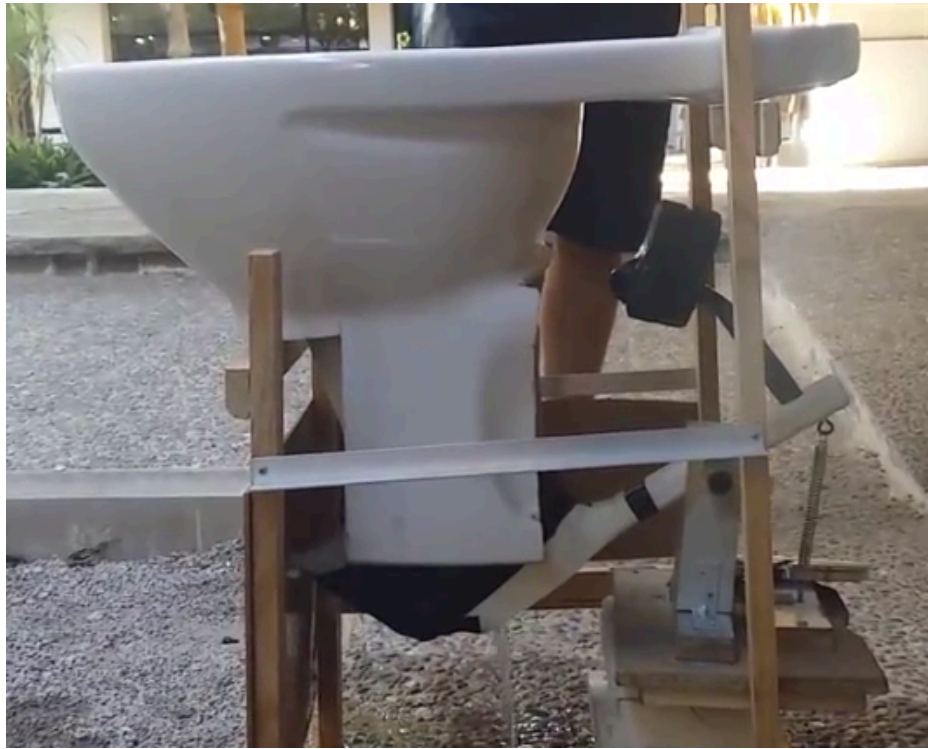
Figure 35. open Flapper at 25° Prototype
