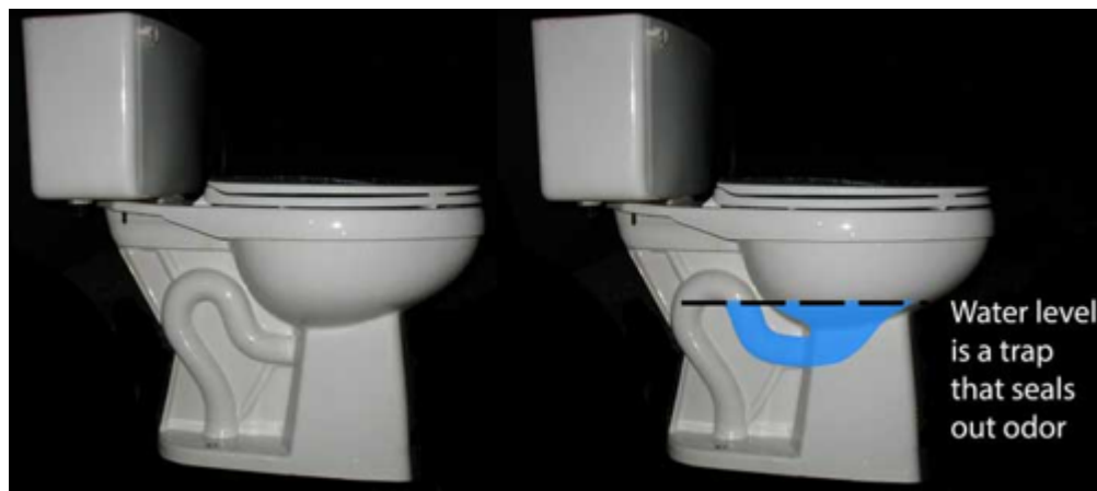
Figure 6. Diagram of Water Trap in Standard Toilet
