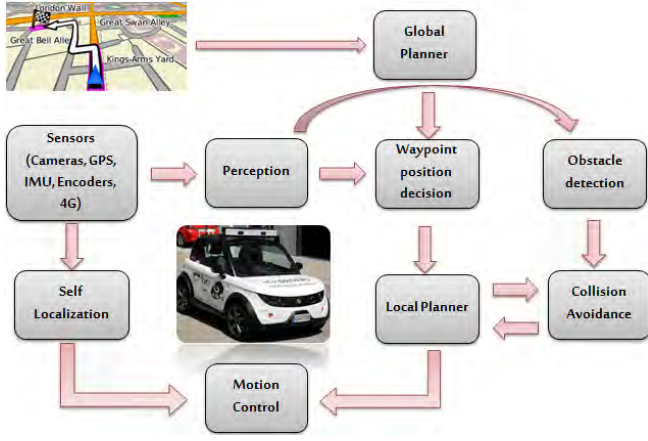
Fig. 2. System architecture of the autonomous vehicle
