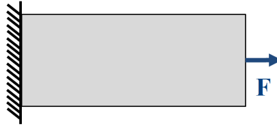
Figure 3: Schematic drawing of a traction rod with homogeneous material distribution
