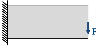
Figure 5: Schematic drawing of a cantilever beam with homogeneous material distribution
