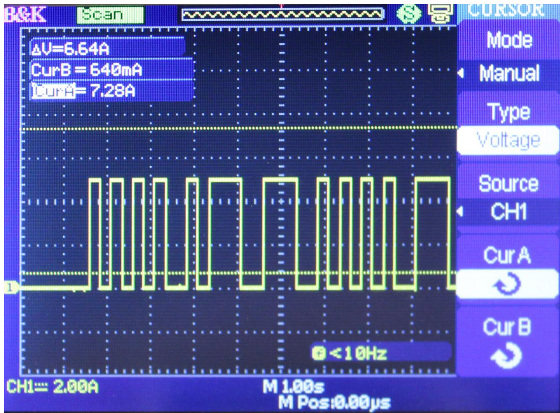
Fig. 9.1 Digital signal with Morse shape, output from an Arduino. HATH... can be deduced, from the heading of the message which includes the name of the satellite: Hathor.
